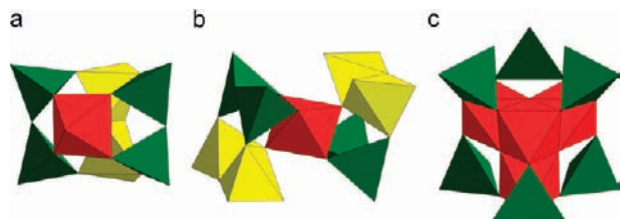
Figure 1. Three of the most common clusters in open-framework germanates. (a) The \text{Ge}_7 cluster. (b) The \text{Ge}_9 cluster. (c) The \text{Ge}_{10} cluster. \text{GeO}_6 octahedra are in red, \text{GeO}_5 trigonal bipyramids in yellow, and \text{GeO}_4 tetrahedra in green.
